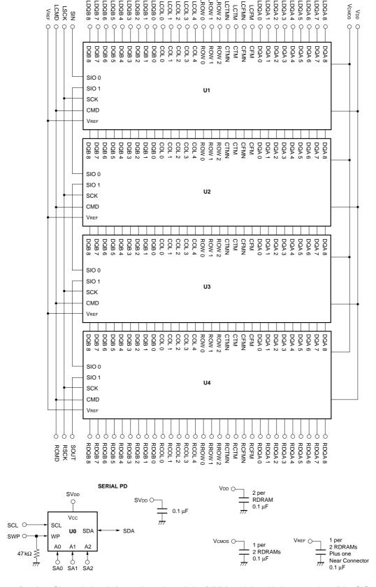
Remarks 1. Rambus Channel signals form a loop through the RIMM module, with the exception of the SIO chain.2. See Serial Presence Detection Specification for information on the SPD device and its contents.
